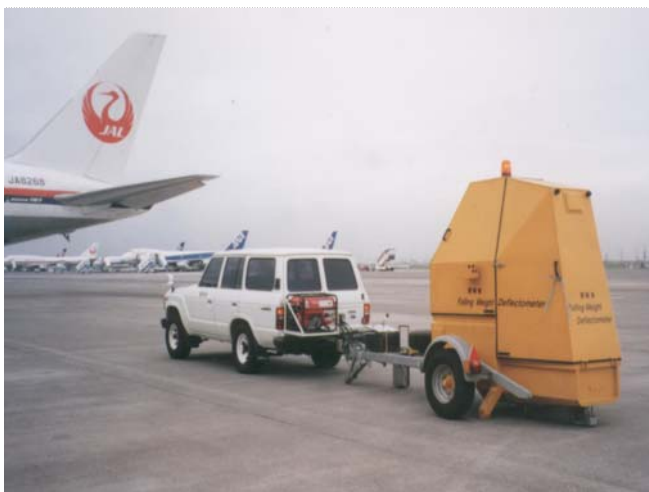
Fig. 4. FWD (Falling Weight Deflectometer).
