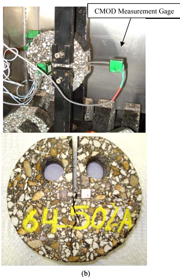
Fig. 2. Experimental Setup for DC(T) Testing (a) DC(T) Test Setup and (b) DC(T) Test Specimen after Test.
