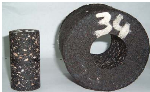
Fig. 2. Triaxial Test Specimen Cored from Marshall Sample.
