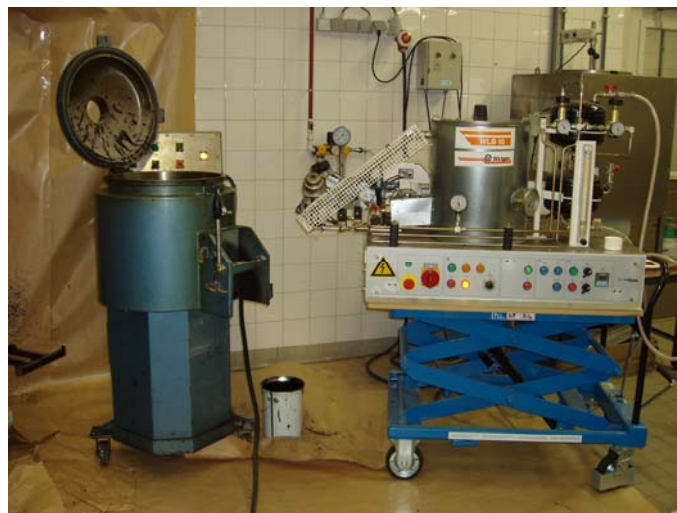
Fig. 1. Wirtgen Laboratory Foam Unit, Together with the Asphalt Mixer.
