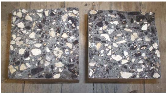
Fig. 2. Typical Fracture Surfaces of Concrete Sample Containing RAP.
