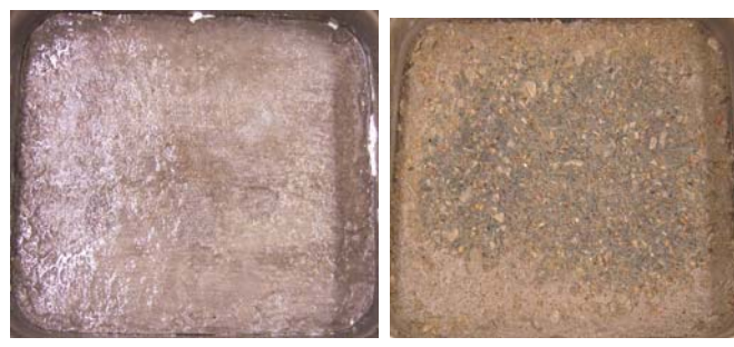
Fig. 16. S-BO-21 After 5 and 50 Deicer Cycles.
