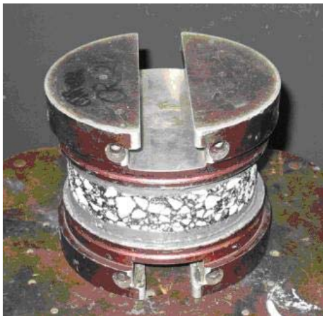
Fig. 5. A Shear Test Specimen Glued to Loading Platens.
