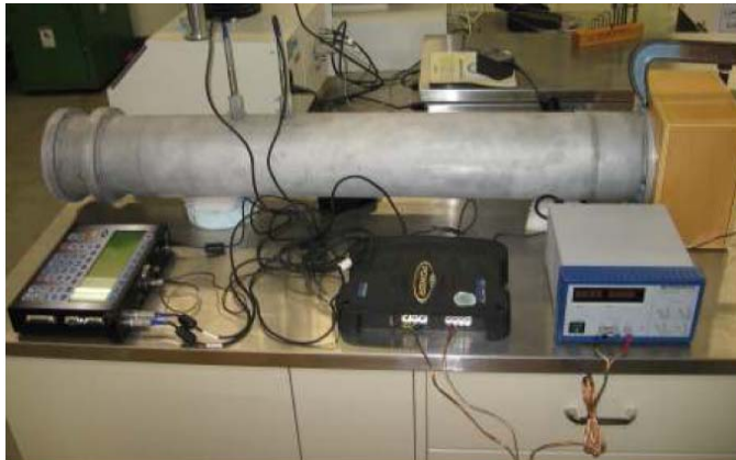
Fig. 3. Impedance Tube for Sound Absorption Testing at CPATT Laboratory.
