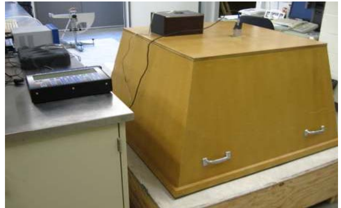
Fig. 4. Sound Absorption Testing using Portable Reverberation Chamber.
