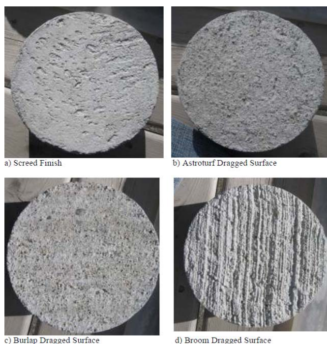
Fig. 1. Sample Pictures of the Textured PCC Surfaces.
