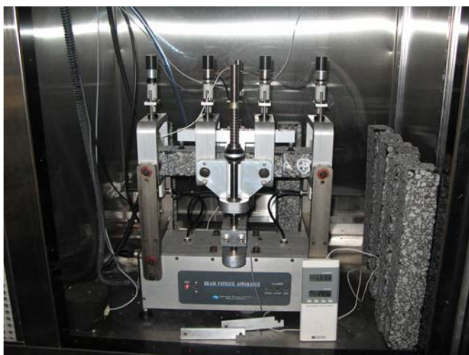
Fig. 2. University of Canterbury Bending Beam Fatigue Apparatus.
