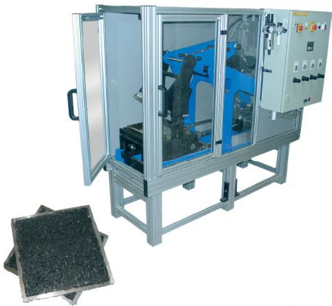
Fig. 1. Downer EDi Works Contractor Roller Compactor.
