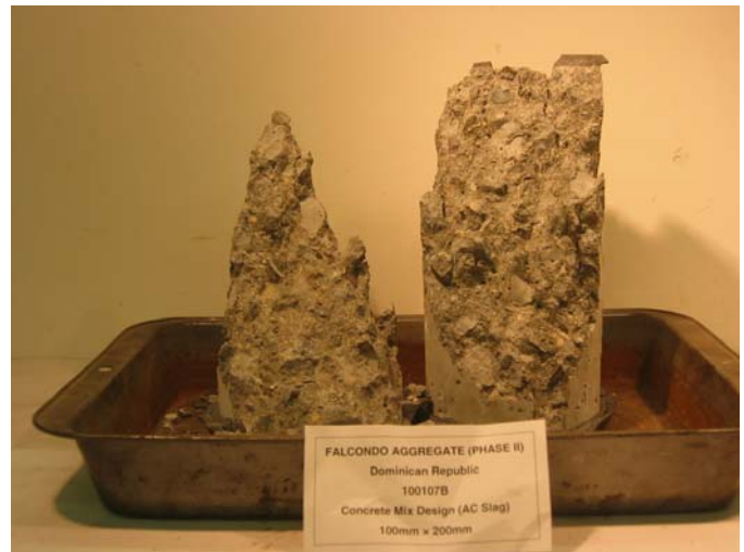
Fig. 4. Concrete Containing Air Cooled Nickel Slag as Coarse Aggregate after Breaking.
