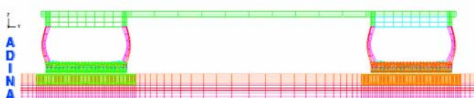
Fig. 8. Contact Surfaces between Tire and Pavement Surface.
