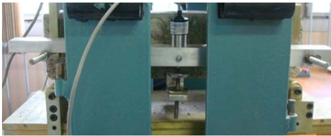
Fig. 5. LVDT Capturing Beam Deflection During Flexural Tensile Test.
