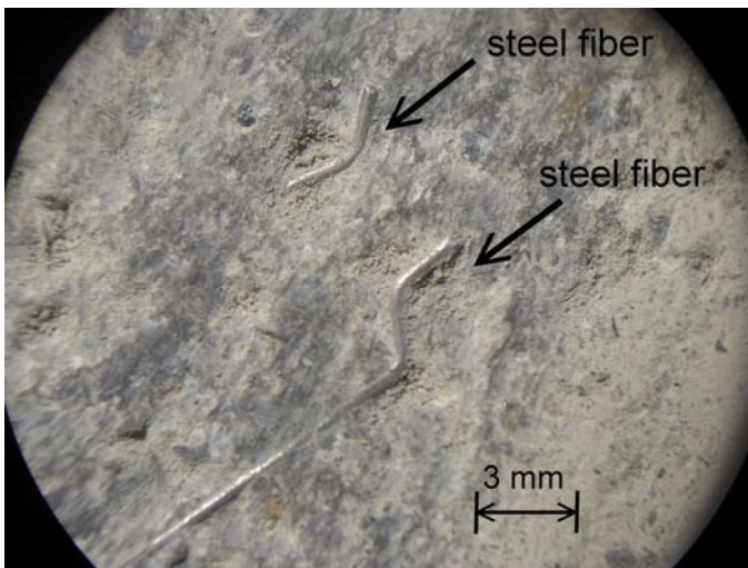
Fig. 3. Specimen Surface of SPHFRC during Final Stage.
