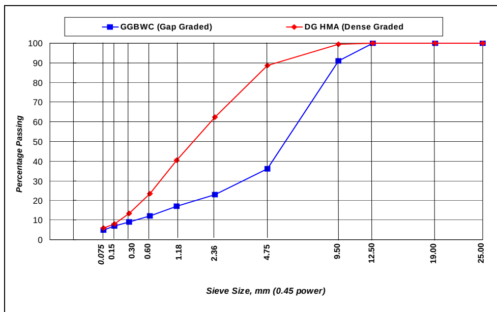
Fig. 1. Aggregate Gradations for Gap-Graded and Dense-Graded Mixtures.
