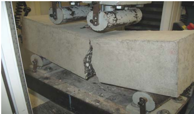
Fig. 1. Failure of Concrete Beam Containing RAP.
