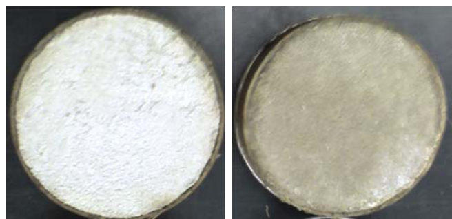
Fig. 2. Samples after Moisture Loss Testing, Without (Left) and With (Right) Soybean Oil.
