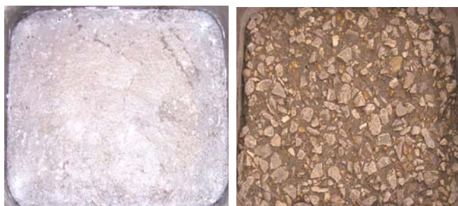
Fig. 11. OPC-BO After 5 and 50 Deicer Cycles.
