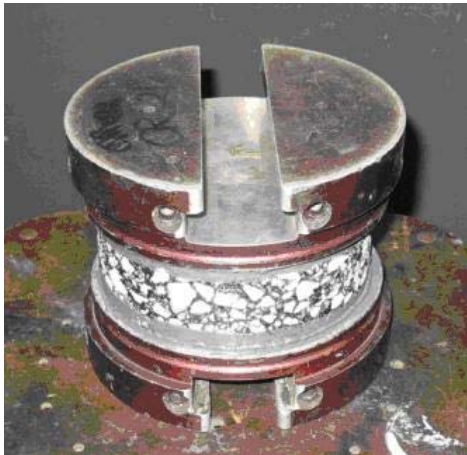
Fig. 5. A Shear Test Specimen Glued to Loading Platens.
