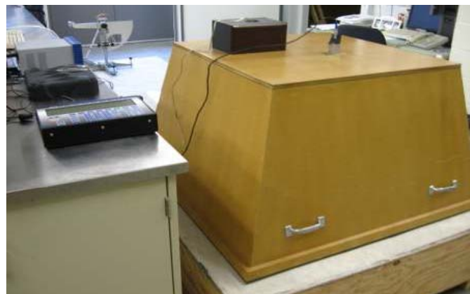
Fig. 4. Sound Absorption Testing using Portable Reverberation Chamber.
