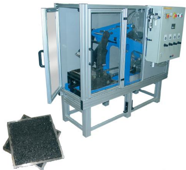
Fig. 1. Downer EDi Works Contractor Roller Compactor.
