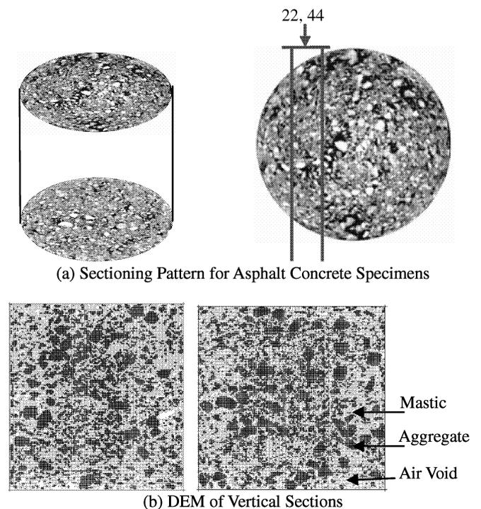
**Fig. 4.** Illustration of Vertical Section from 3D Image.
