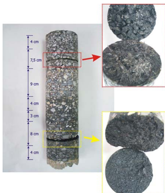
Fig. 5. Cores (diameter 10 cm) Collected in 2009. a) Core 2a Collected at the Right-hand-side Wheel Track, in Which the Lack of Bonding between Upper and Lower Bonding Layers is Visible; b) Core 2b Collected in the Center of the Hard Shoulder – the Bonding of Layers has been Visually Assessed as Good.
