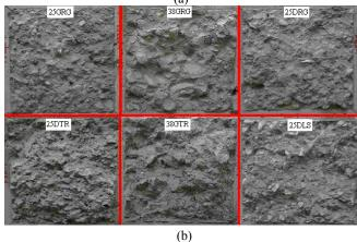
**Fig. 5.** (a) Wedge Split Test Specimen Setup; (b) Cracked Surfaces of the Tested Specimens.
