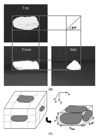
**Fig. 2.** (a) Three Orthogonal Views of a Particle Captured by the UIAIA; (b) Smallest Rectangular Framework Determined for Containing an Aggregate Particle.
