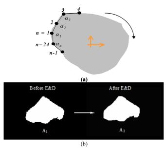
**Fig. 1.** (a) Illustration of An *n*-sided Polygon Approximating the Outline of an Aggregate Particle; (b) Change of the Particle Surface Texture before and after the Optimum Cycles of Erosion and Dilation.
