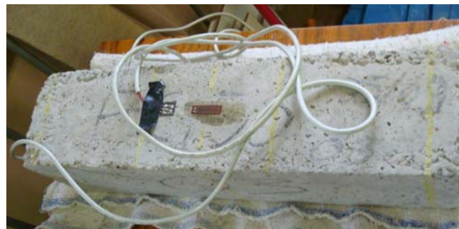
Fig. 6. Strain Gage Attached to Beam Bottom to Achieve Flexural Maximum Strain During Test.
