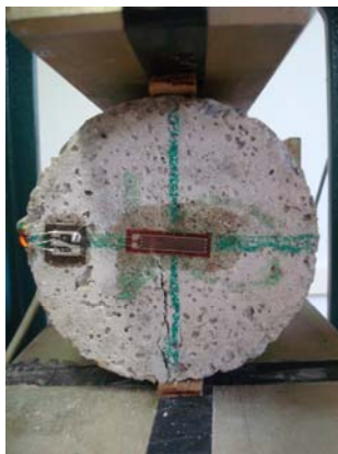
Fig. 4. Split Test with Horizontal Maximum Strain Measurements of RCC Sample.
