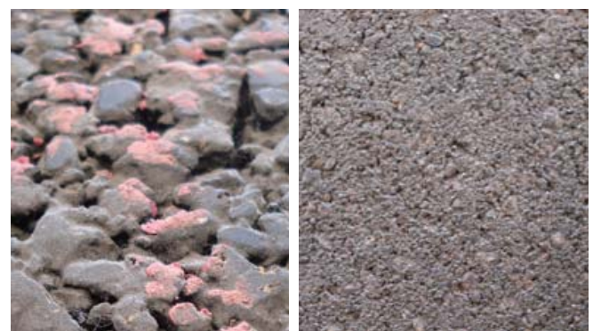
Fig. 4. Texture of SMA (Left) and Conventional Mix (Right) (after [6]).
