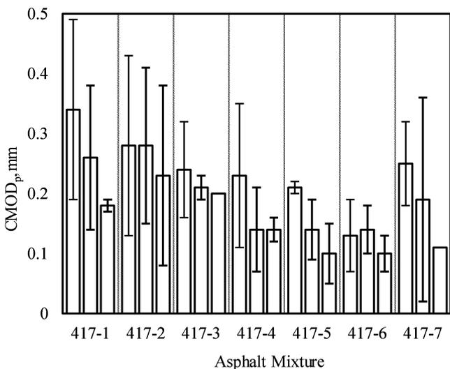
**Fig. 4.** Crack Mouth Opening Displacements at Peak Load after Various Conditioning Times.
