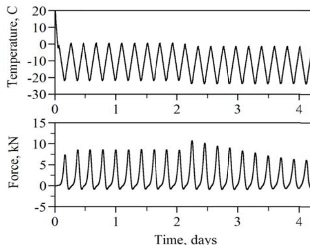
**Fig. 1.** Thermal Fatigue Cycles on Asphalt Mixture Sample [32]. *Note:* First ten cooling cycles incurred no damage while second ten cycles were just below the damage threshold of  $-22^{\circ}\text{C}$ .
