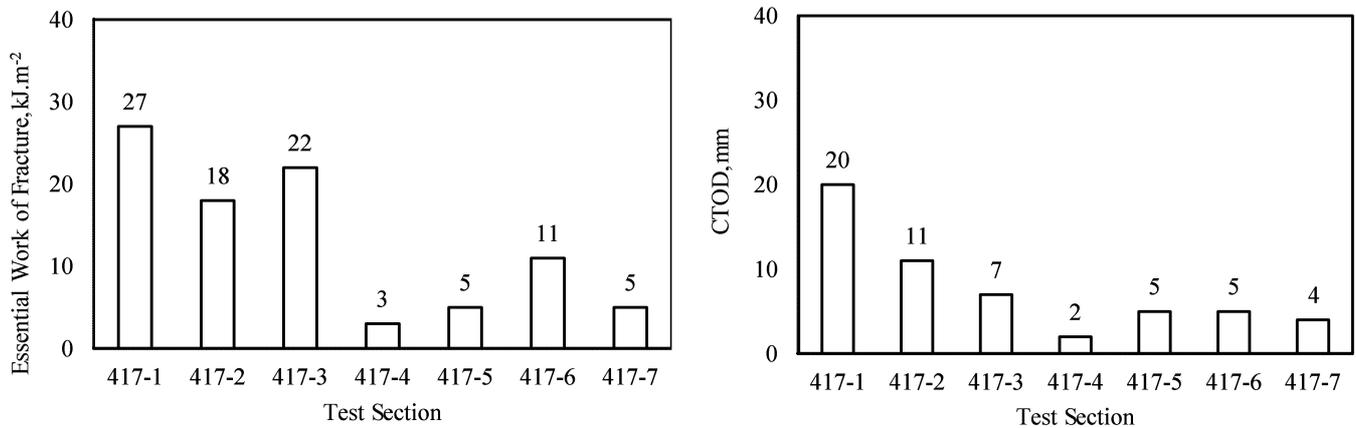
**Fig. 2.** (a) Essential Works of Fracture for Asphalt Cements; and (b) Approximate Critical Crack Tip Opening Displacements for Asphalt Cements (T = 15°C).
