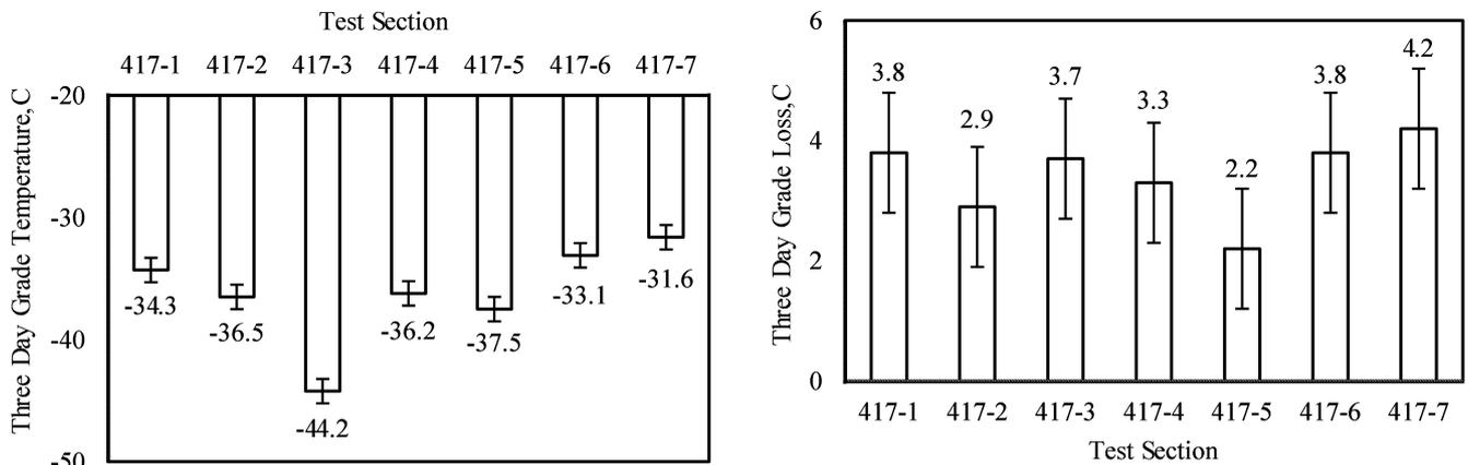
**Fig. 3.** Extended BBR Test Results: (a) Absolute Grade after Three Days Conditioning at -20°C; and (b) Grade Loss after Three Days of Conditioning.
