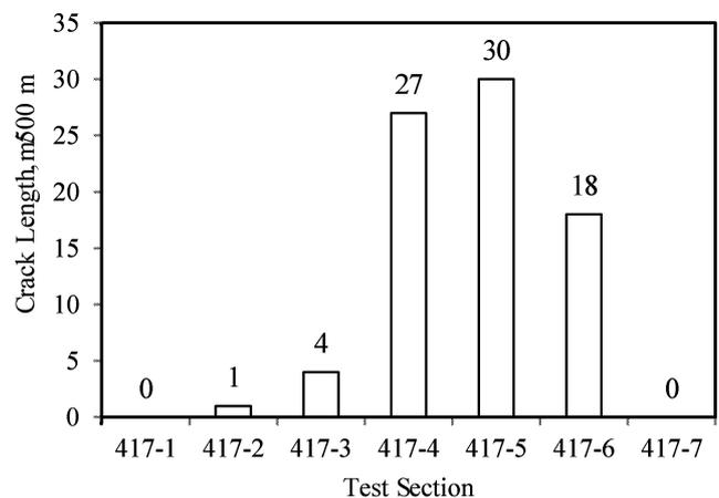
**Fig. 7.** Pavement Distress for Summer 2010: (a) Number of Cracks for Each Section; and (b) Total Crack Length for Each Section.
