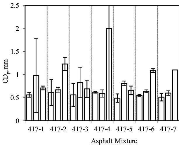
**Fig. 5.** Crosshead Displacements at Peak Load after Various Conditioning Times.
