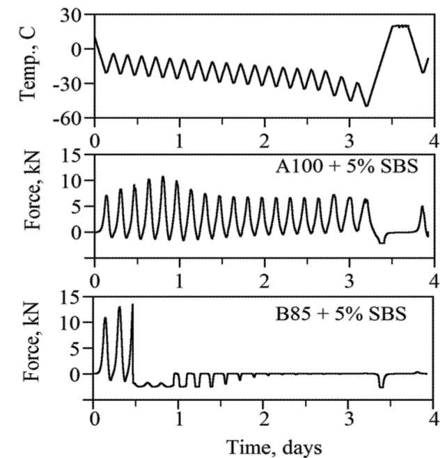
**Fig. 6.** Thermal Fatigue Cycles on Asphalt Mixture Samples [32].
