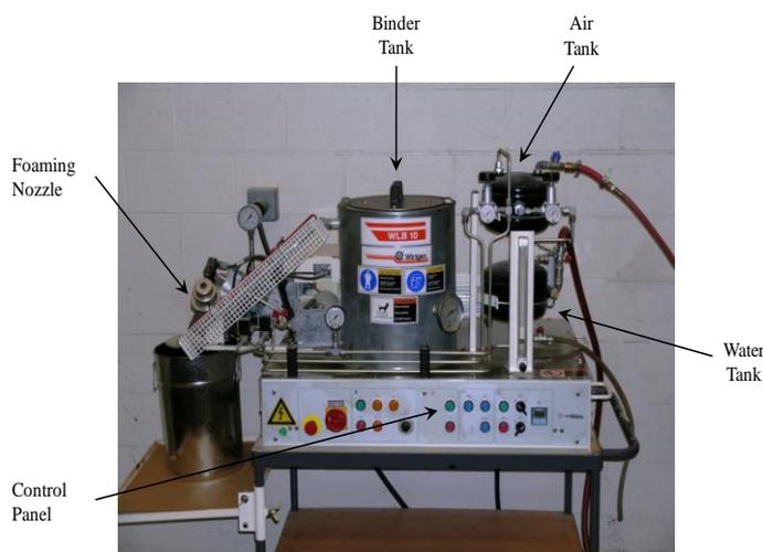
**Fig. 2.** Laboratory Asphalt Foaming Device.
