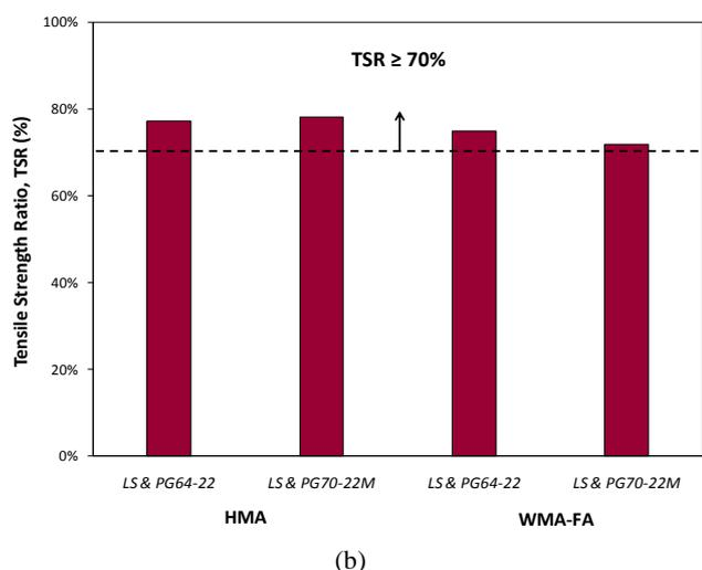
**Fig. 5.** Moisture Susceptibility Test Results: a. Gravel, b. Limestone.
