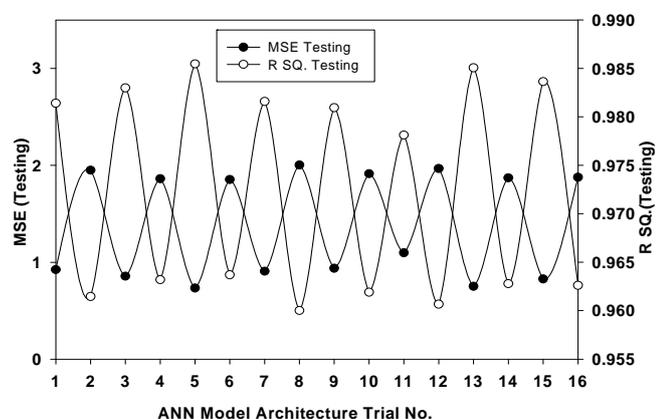
**Fig. 6.** Variation in MSE and R SQ. for the Rut-depth Progression ANN Model (Suggested Model Architecture No. 5)
