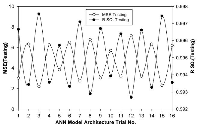
**Fig. 4.** Variation in MSE and R SQ. for the Raveling Progression ANN Model (Suggested Model Architecture No. 3)
