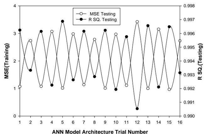
**Fig. 3.** Variation in MSE and R SQ. for the Cracking Progression ANN Model (Suggested Model Architecture No. 15)
