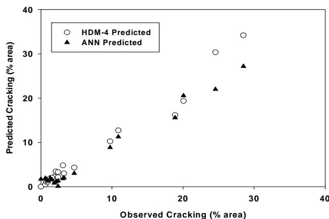
**Fig. 7.** Scatter Plot of Observed Distresses vs. HDM-4 and ANN Model Predicted Cracking.
