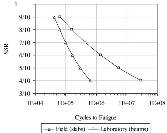
**Fig. 7.** Field and Laboratory Fatigue Curves of the Investigated Concrete.
