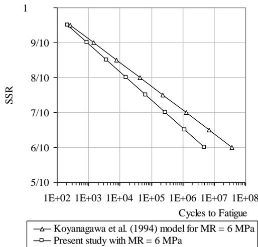
**Fig. 6.** Results for the Logarithmic Regression Fatigue Model of Constant Stress.
