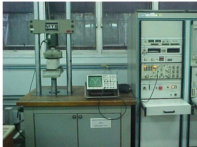
**Fig. 1.** Servo-controlled Machine for Fatigue Tests.
