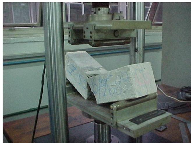
**Fig. 2.** Half-span Rupture of Concrete.
