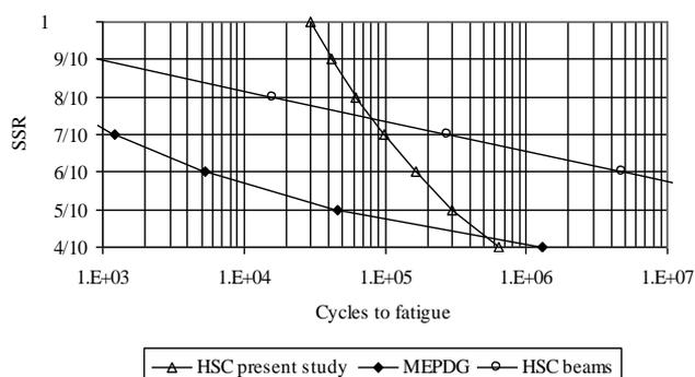
Fig. 10. Comparison of HSC Fatigue Functions to MEPDG.
