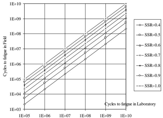
**Fig. 8.** Cycles to Fatigue in the Field and for Beams as a Function of the Stress-strength Ratio (SSR).
