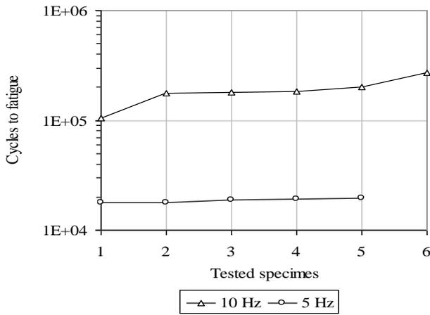
**Fig. 5.** Cycles to Fatigue Due to Different Load Application Frequencies for SSR = 0.73.
