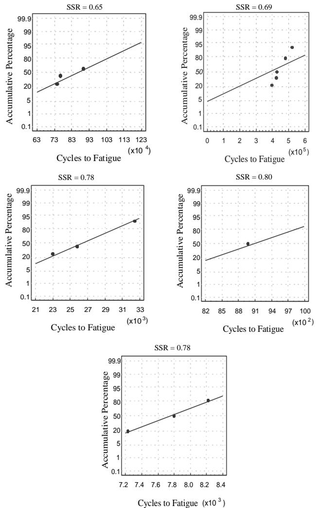
**Fig. 4.** Failure Probability for Several SSR Levels (According to K-S Test).
