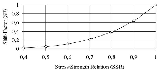
Fig. 9. Shift-Factor as a Function of SSR.
