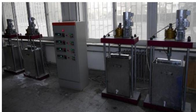
Fig. 7. Mechanical Corrosion Fatigue System.
