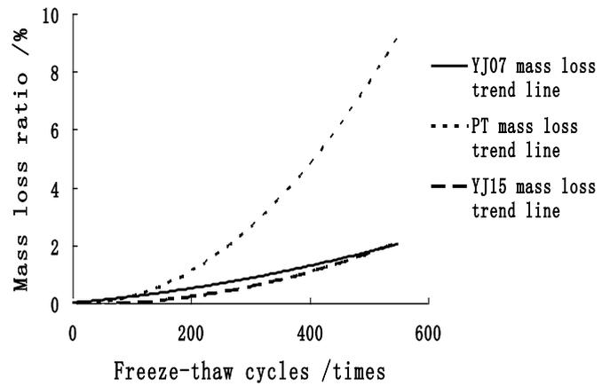
Fig. 4. Effects of Freeze-thaw Cycles on the Mass Loss of the Concrete Pavement.
