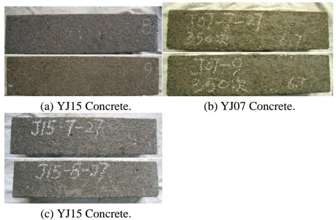
Fig. 5. Concrete Specimens: (a) after 300 freeze-thaw cycles, mass loss ratio: 0.4%(0.21kg/m<sup>2</sup>); (b) after 350 freeze-thaw cycles, mass loss ratio: 1.0%(0.60kg/m<sup>2</sup>); (c) after 550 freeze-thaw cycles, mass loss ratio: 2.0%(1.05kg/m<sup>2</sup>).
