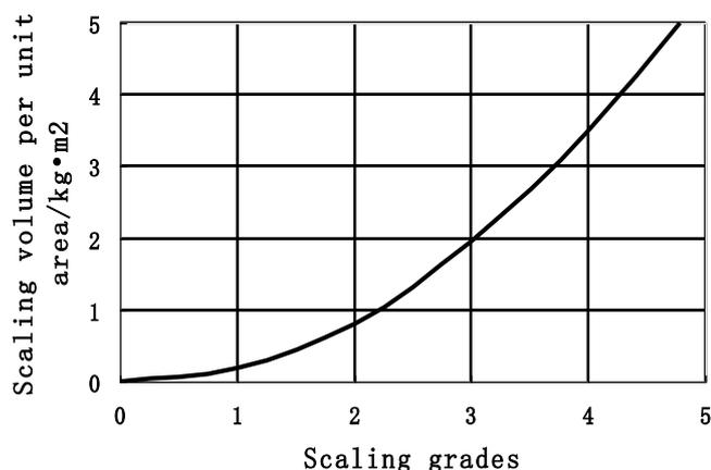
**Fig. 2.** Correlation between the Deicer-scaling Grade and Scaling Volume Per Unit Area [6].
