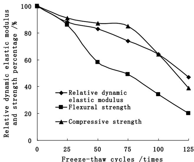
**Fig. 1.** Effects of Freeze-thaw Cycles on the Strength of Concrete [3].
