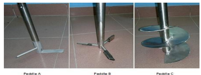
Fig. 2. Photograph of Three Types of Paddle Used in Research.
