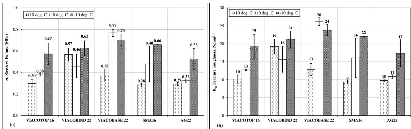
Fig. 5. SCB Test Results for The Field-cored Mixes for the Different Layers: (a)  $\sigma_f$ , Stress at Failure; (b)  $K_{IC}$ , Fracture Toughness (Stress Intensity Factor).
