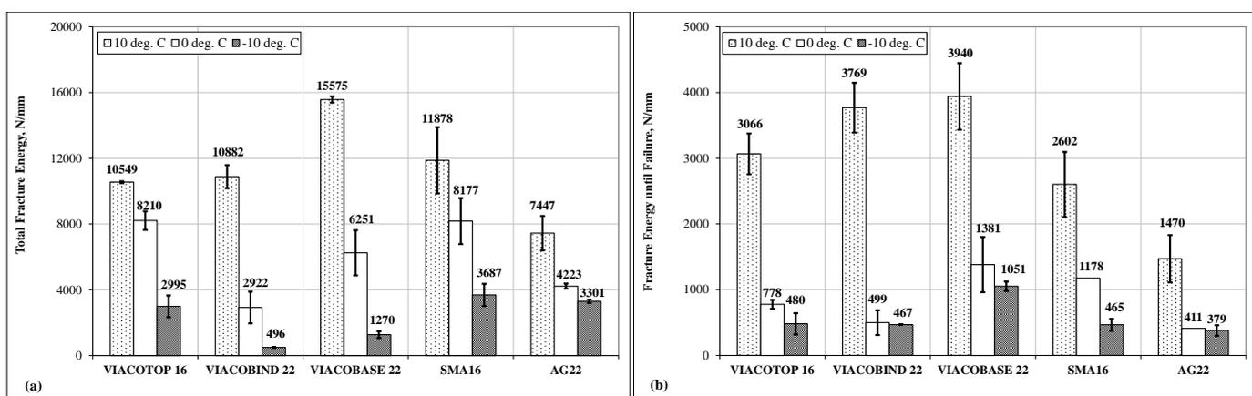
Fig. 6. SCB Test Results for The Field-cored Mixes for The Different Layers: (a) Total Fracture Energy; (b) Fracture Energy Until Failure.
