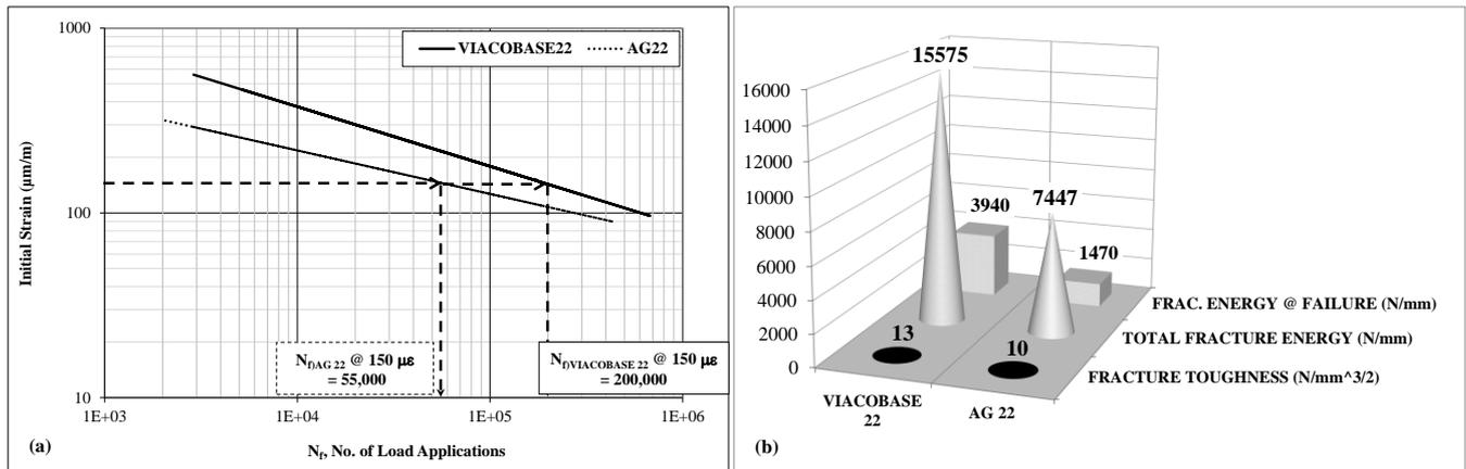
**Fig. 7.** (a) Fatigue Relationships for VIACOBASE 22 and AG 22 Estimated from Fatigue Tests at 10°C [12]; (b) Fracture Characteristics for VIACOBASE 22 and AG 22 from SCB Tests.
