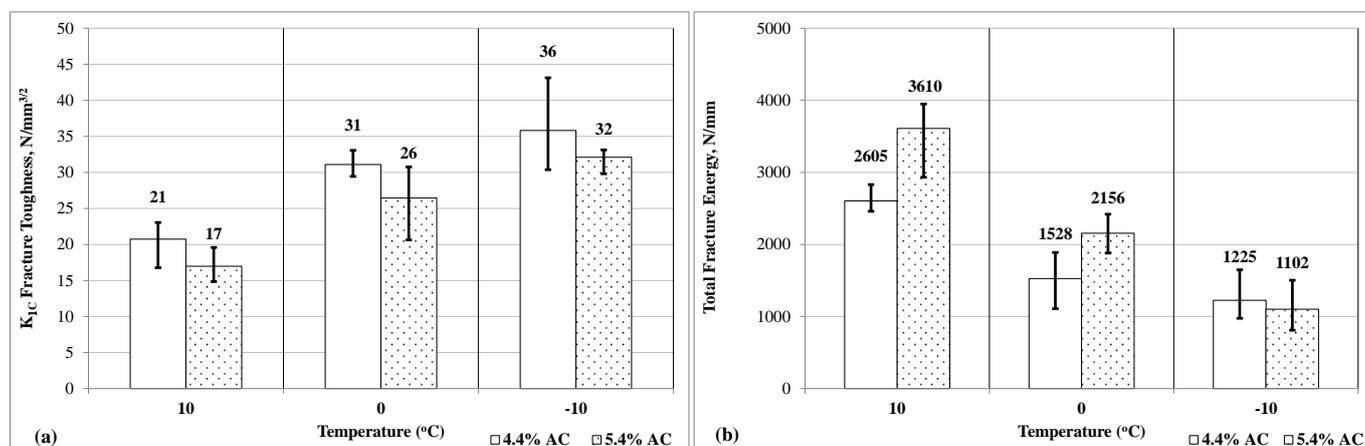
Fig. 3. SCB Test Results for The Laboratory Blended Mixes: (a)  $K_{1C}$ , Fracture Toughness (Stress Intensity Factor) (b) Total Fracture Energy.
