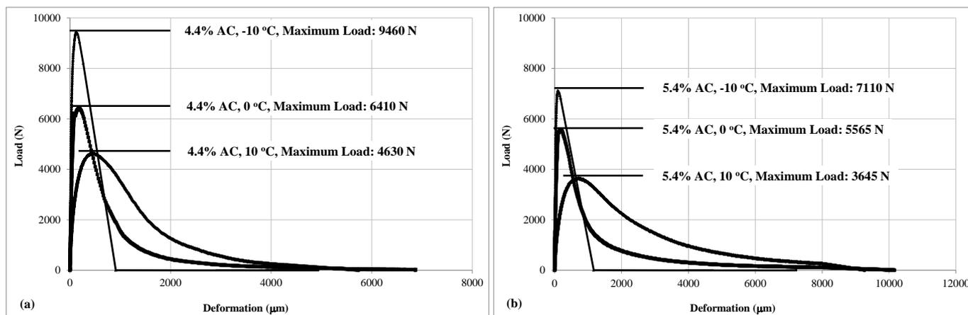
Fig. 2. Load–Deformation Relationships for Laboratory Blended Mixes at Different Temperatures for: (a) 4.4% Asphalt Content (b) 5.4% Asphalt Content.
