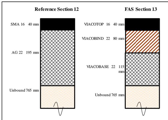
**Fig. 4.** Pavement Structures of the Reference and the FAS Road Sections on The Swedish E6 Highway [12].
