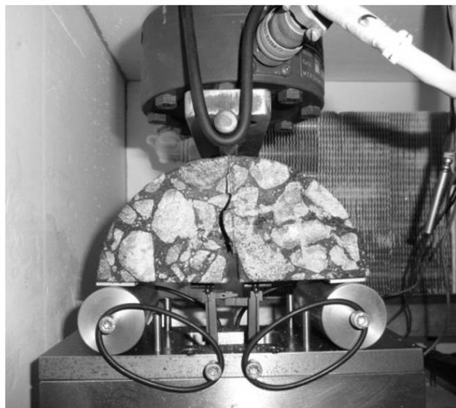
**Fig. 1.** Actual Semi-circular Bending Test Setup; The Sample Also Shows Cracks That Initiated at The Tip of The Notch and Propagated to The Top of The Specimen During The Experiment.
