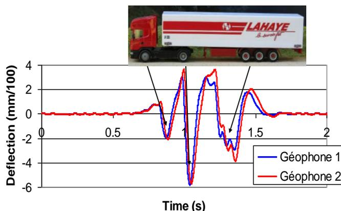
**Fig. 11.** Integrated Signal of Geophone Under a Five-axle Truck.
