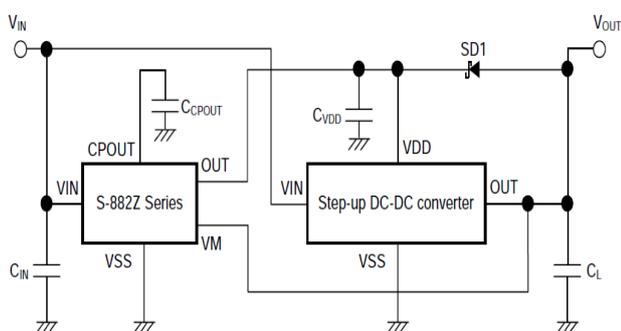
Fig. 5. Connection Diagram for the Circuit Design of the Energy Harvesting System.
