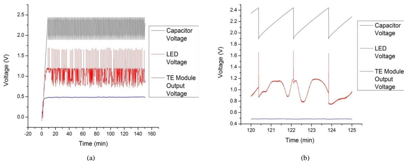
Fig. 8. a) Voltage at the TE Element, Capacitor and LED, b) Zoom in between 120 to 125 min.
