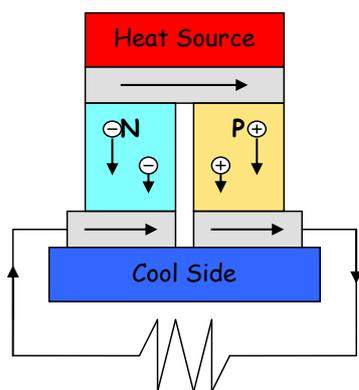
Fig. 4. A Thermoelectric Module Used as a Power Generator.
