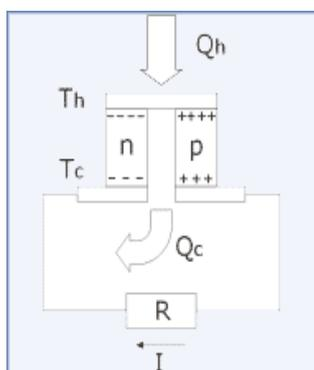
Fig. 3. Schematic of Thermoelectric Generator Principle.
