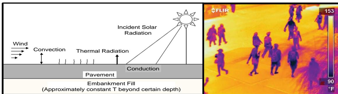
Fig. 1. a) Thermal Balance at the Surface of Road; b) Pavement Surface Temperature by Infrared Camera (EPA 2009)[2].
