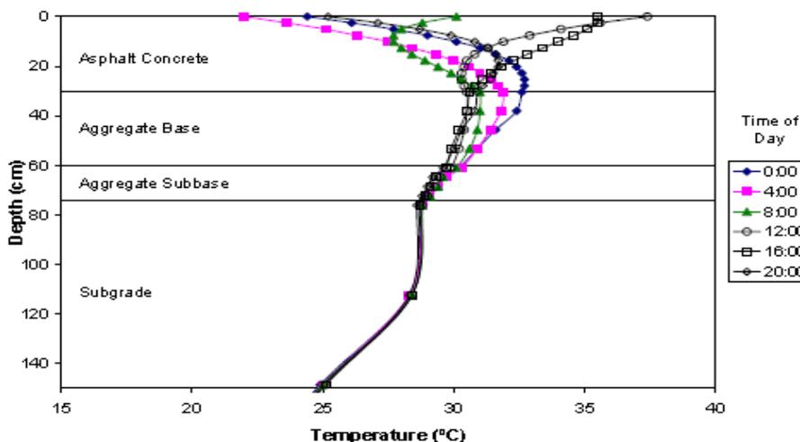
Fig. 2. Example Measured Daily Temperature Variations under Pavement (Ongel and Harvey 2004 [3]).
