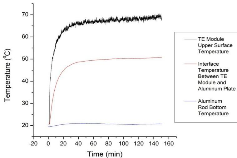
Fig. 7. Monitored Temperature Process at Different Locations in the Thermal Energy Harvesting System.
