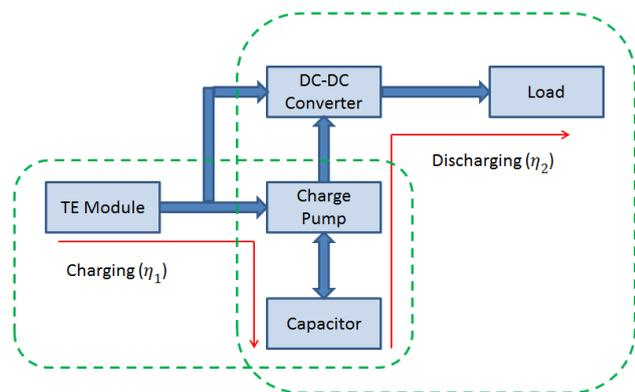
Fig. 9. Energy Flow in the Energy Harvesting System Circuit. ( $\eta_1$  is the Efficiency when The Capacitor is Charging.  $\eta_2$  is the Efficiency when the Capacitor is Discharging).
