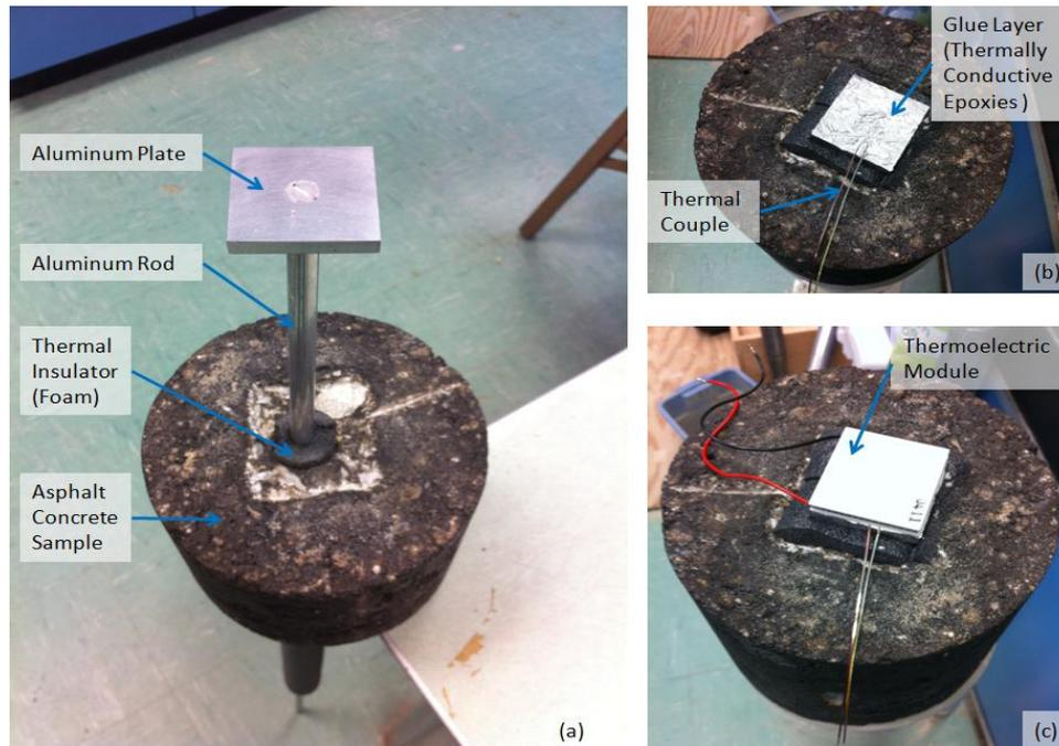
Fig. 6. Illustration of Thermal Harvesting System Set up.
