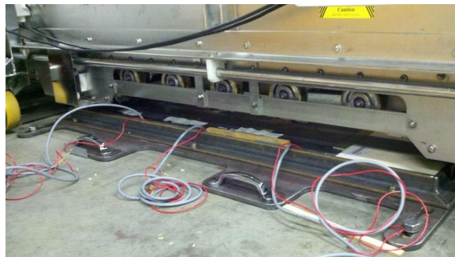
Fig. 7. Model Mobile Lading Simulator laboratory testing frame.
