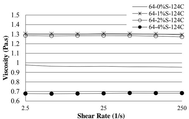
Fig. 6. Effects of Shear Rate at 64°C, 100°C and 124°C on PG 64-22 with Sasobit®.
