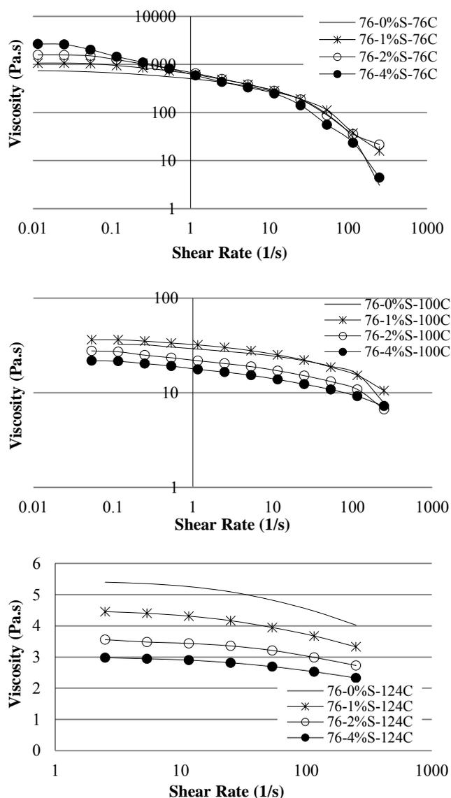
**Fig. 7.** Effects of Shear Rate at 76°C, 100°C and 124°C on PG 76-22M with Sasobit®.
