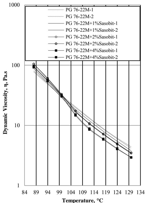
**Fig. 3.** Dynamic Viscosity,  $\eta$  (Pa.s) of PG 76-22M at Compaction Temperatures.
