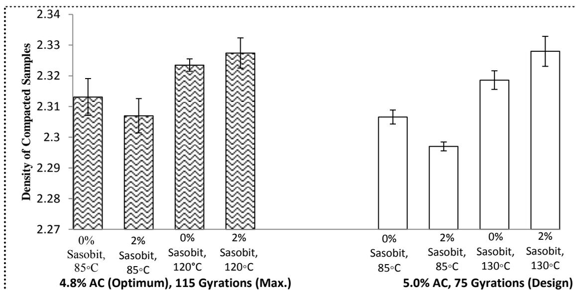
Fig. 4. Effect of Sasobit® on Density of Gyrotary Compacted Samples.
