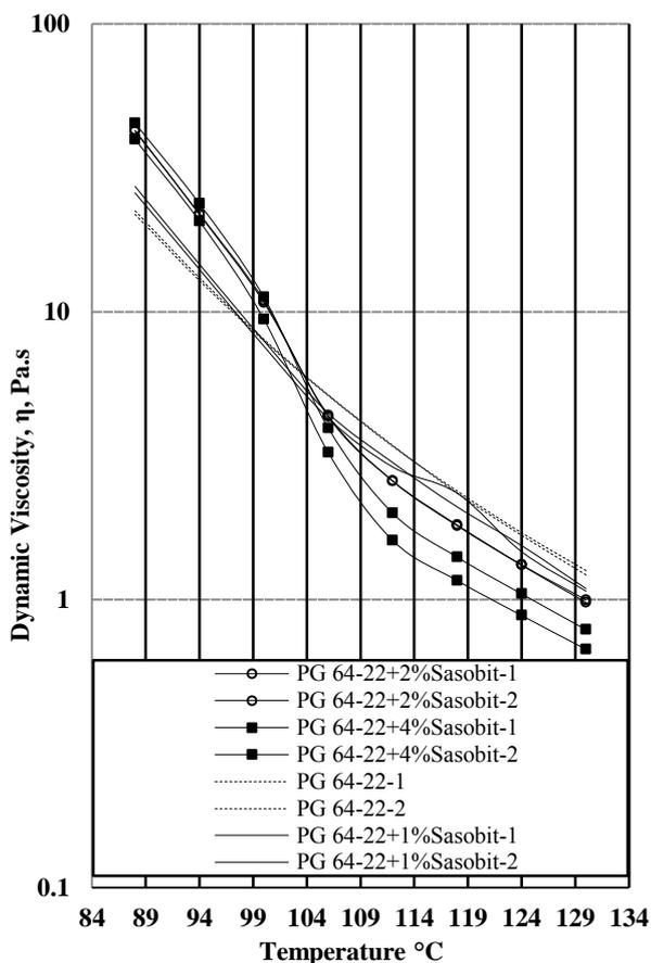
**Fig. 2.** Dynamic Viscosity,  $\eta$  (Pa.s) of PG 64-22 at Compaction Temperatures.
