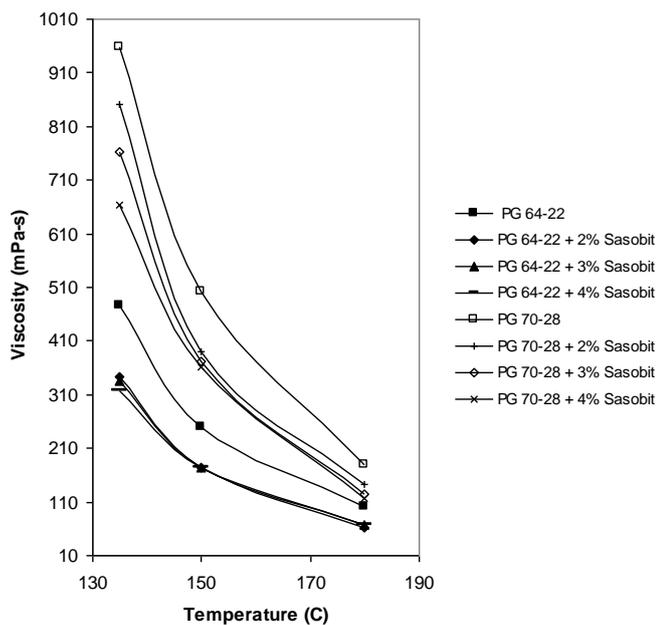
**Fig. 1.** Rotational Viscosity of PG64-22 and PG70-28 (Reproduced from Wasiuddin *et al.* [8]).
