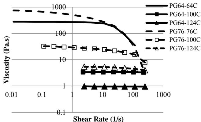
Fig. 5. Effect of Temperature on Shear Rate Dependency.
