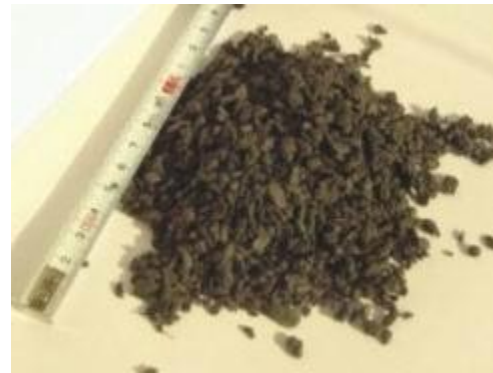
Fig. 1. Modifier used in the Study - Duroflex ®
