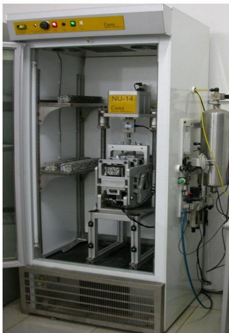
Fig. 5. Cooper NU-14 Four-Point Bending Tester.
