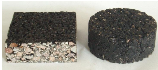
Fig. 4. Square and Circular Samples for the Cone Calorimeter Test.
