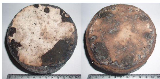
Fig. 6. Samples of W-550A (Right) and W-550C (Left) Asphalt Mixtures After Cone Calorimeter Test. Top Surface.
