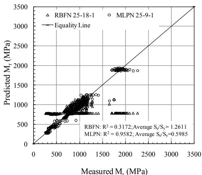
**Fig. 7.** Predicted Mr Versus Measured Mr for K-soil Using RBFN 25-18-1 and MLPN 25-9-1 Neural Network Models.
