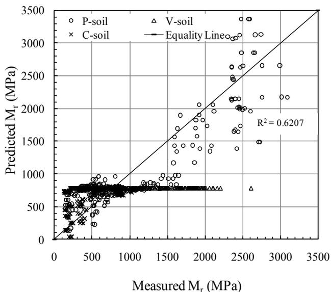
Fig. 2. Predicted Mr Versus Measured Mr for P-, V- and C-soil using RBFN 25-18-1 Neural Network Model.
