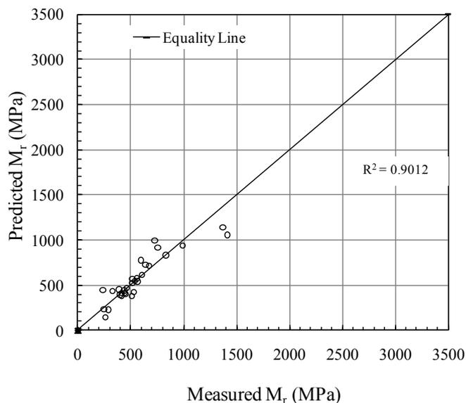
Fig. 3. Predicted Mr Versus Measured Mr for Two Mr Tests: 3% lime-stabilized P-soil and 5% CKD-stabilized V-soil using RBFN 25-10-1 Neural Network Model.
