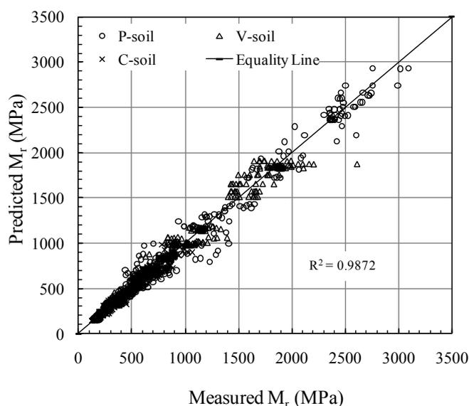
**Fig. 6.** Predicted Mr Versus Measured Mr for P-, V- and C-soil using MLPN 25-9-1 Neural Network Model.
