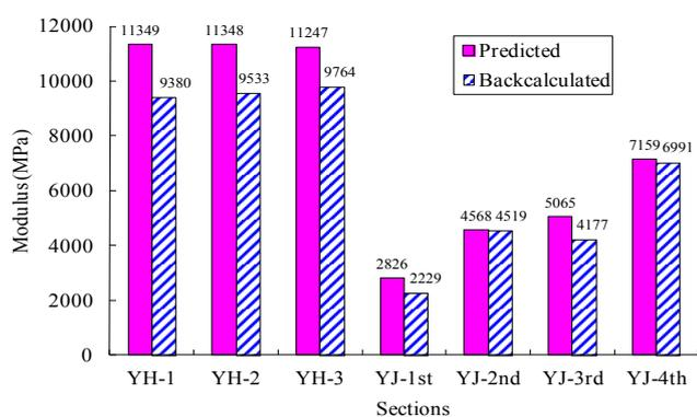
**Fig. 7.** Comparison of the Backcalculated Modulus and the Predicted Modulus  $|E^*|_{equ}$ .
