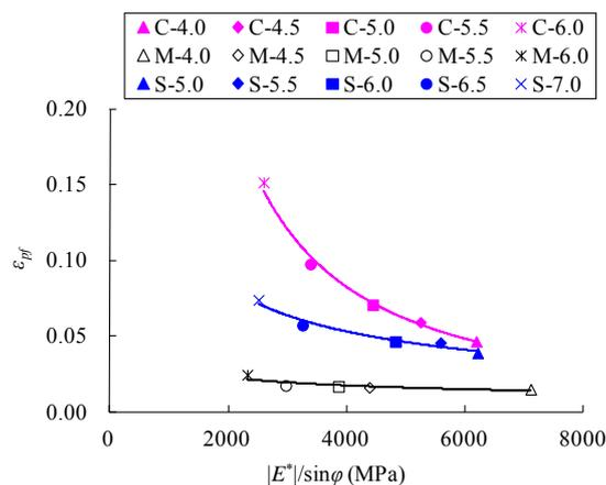
**Fig. 4.** Relation of  $\epsilon_{pf}$  and  $|E^*|/\sin\phi$  at a Temperature of 50°C.
