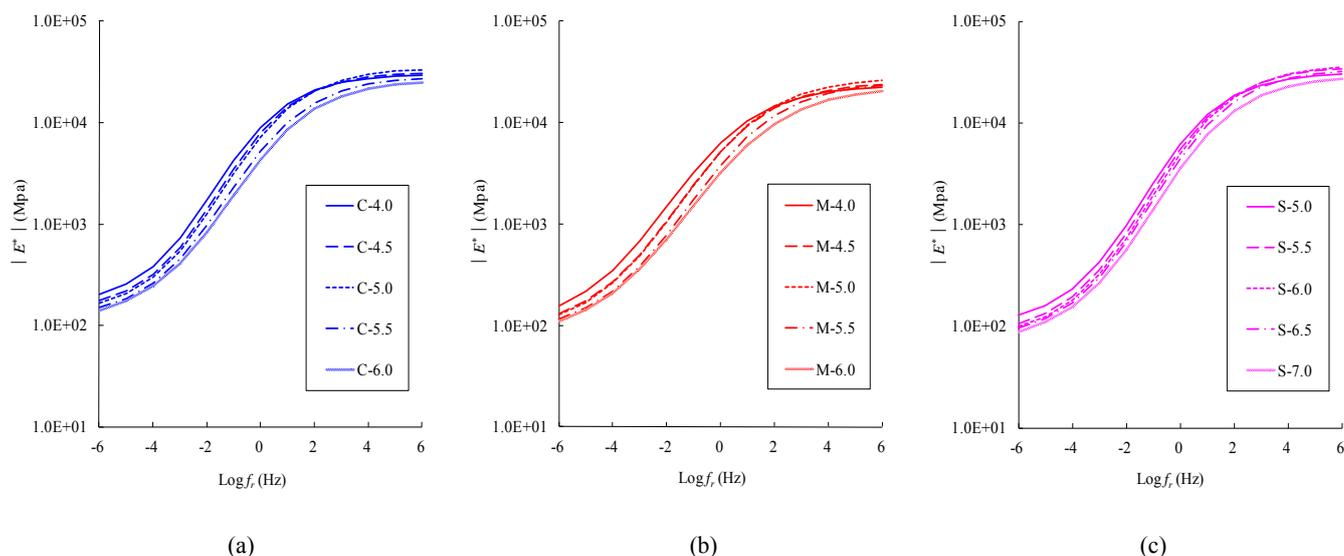
**Fig. 3.** Dynamic Modulus Master Curves for (a) AC-19C, (b) AC-19M, and (c) SMA-13C.
