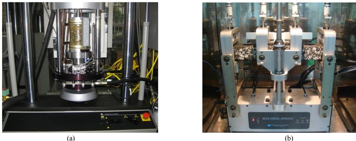
**Fig. 2.** Tests Setup for (a) Dynamic Modulus and RLPD Tests and (b) 4PB Beam Fatigue Test.
