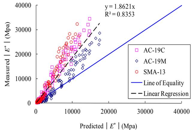
**Fig. 6.** Comparison of the Measured and Predicted  $|E^*|$  Using the Witczak Model.
