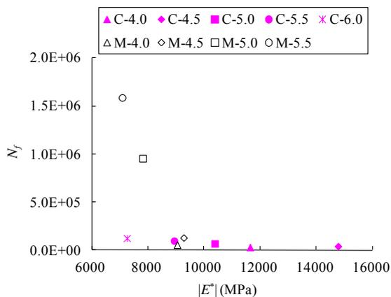
**Fig. 5.** Relation of  $N_f$  and  $|E^*|$  at a Temperature of 20°C.
