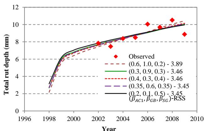
Fig. 2. Predicted Total Rut Depth Curves with Different Combinations of Calibration Parameters.
