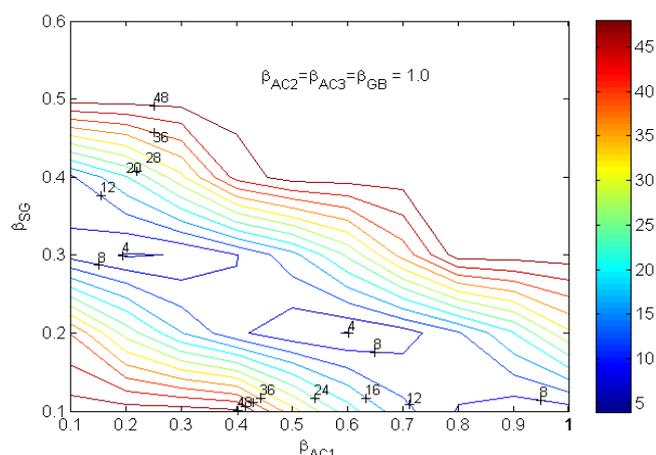
Fig. 1. RSS Contours Against  $\beta_{AC1}$  and  $\beta_{SG}$  Dhowing Multiple Local Minima.
