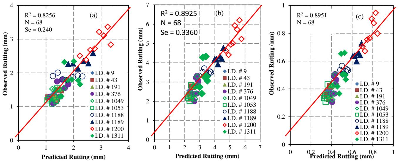
**Fig. 6.** After- section-by-section Calibration Prediction Versus Observation Plots. (a) Asphalt Concrete Layer; (b) Granular Layer (c) Subgrade Layer.
