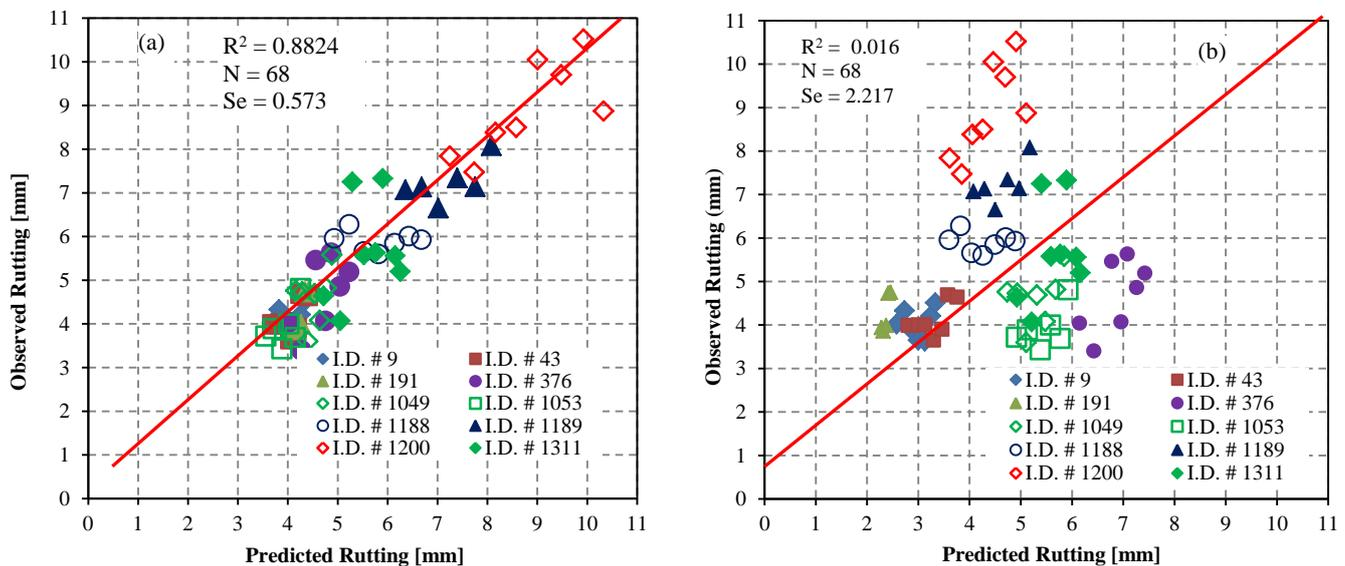
**Fig. 5.** After-calibration Prediction Versus Observation Plots. (a) Section-by-section Calibration; (b) Pooled Calibration.
