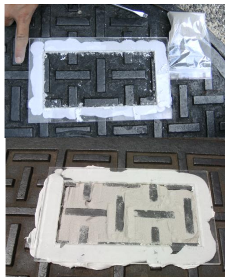
Fig. 4. Applying NTU Improved Sand Patch Method on a Iron-casted Cover.
