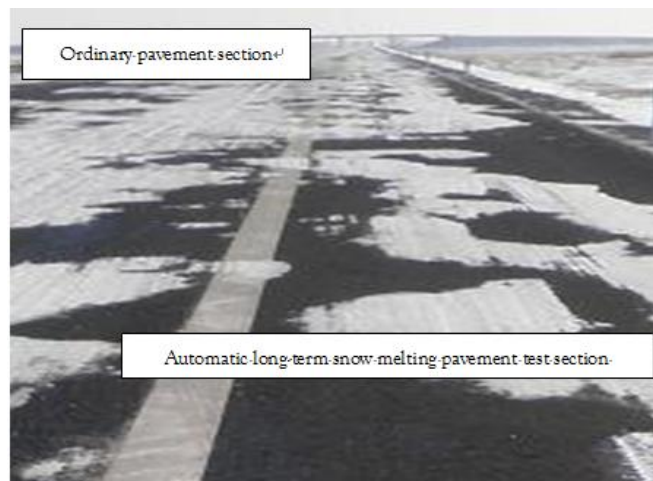
Fig. 9. Deicing Effect of the Automatic Long-term Snowmelt Pavement Test Section.
