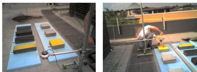
Fig. 4. Roof Positioning and Pyranometer Measurements.
