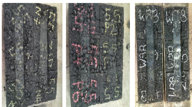
(a) Sample using normal binder (b) Sample using PMB (c) W3B mix
