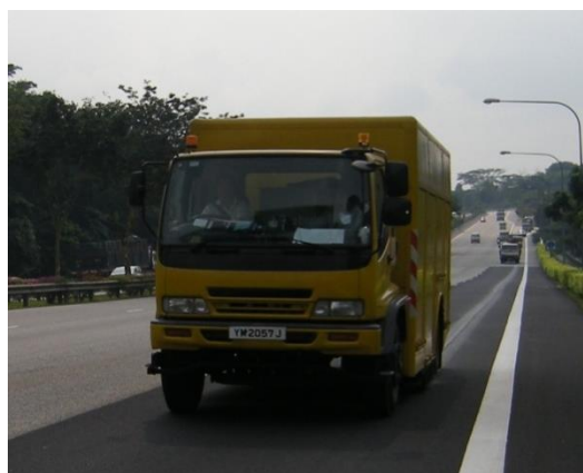
(a) SCRIM machine for measurement of SFC
