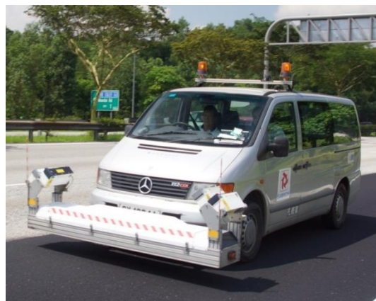
(b) Laser Profiler for measurement of IRI
