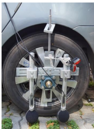
(c) OBSI configuration for measurement of tyre-pavement noise
