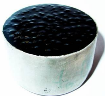
Fig. 2. Heterogeneous Aspect of the Bitumen Modified with SBS Granules (Poor Digestion in Bitumen).
