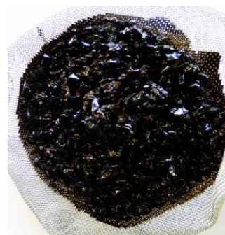
Fig. 3. Granular Particles of ABS That were not Digested Into the Bitumen (Recovered after Filtering the Modified Binder).
