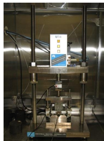
Fig. 2. IDT Test Setup.
