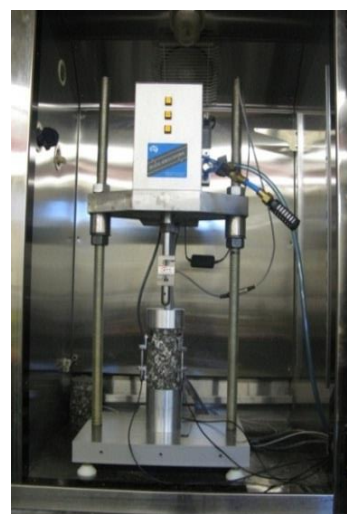
Fig. 1. Uniaxial Compression Test Setup.
