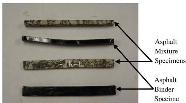
Fig. 1. Preparation of Asphalt Mixture Beam.
