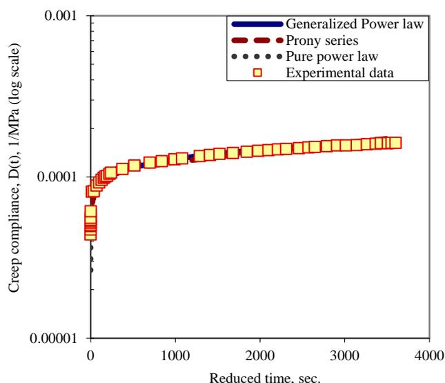
(a) Fitting results based on log creep compliance versus normal time scale
