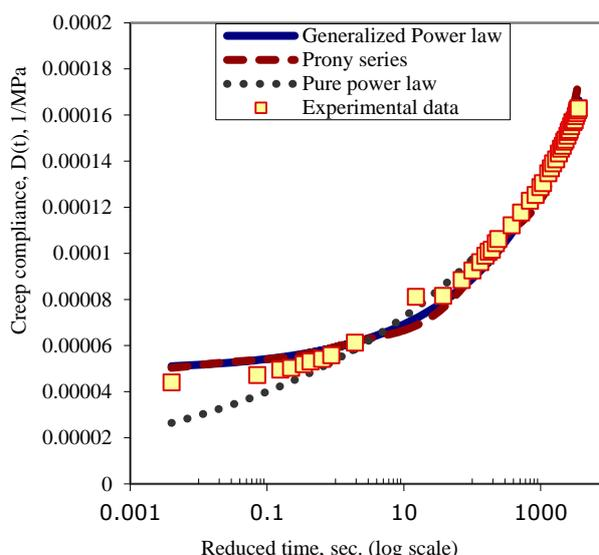
(b) Fitting results based on normal creep compliance scale versus log time scale
