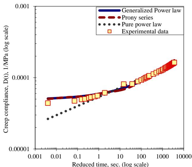
(c) Fitting results based on log creep compliance scale versus log time scale
