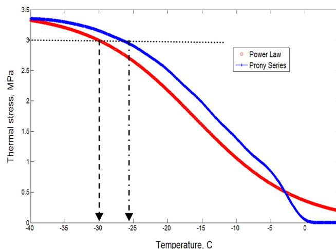
**Fig. 6.** Critical Thermal Cracking Temperatures.
