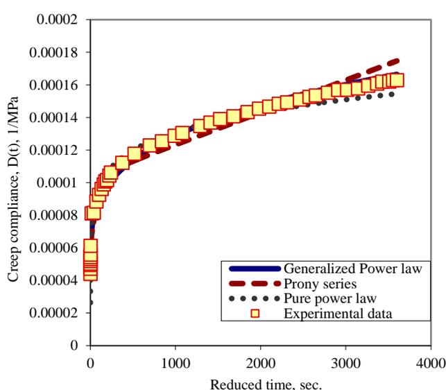
(d) Fitting results based on normal creep compliance scale versus normal time scale
