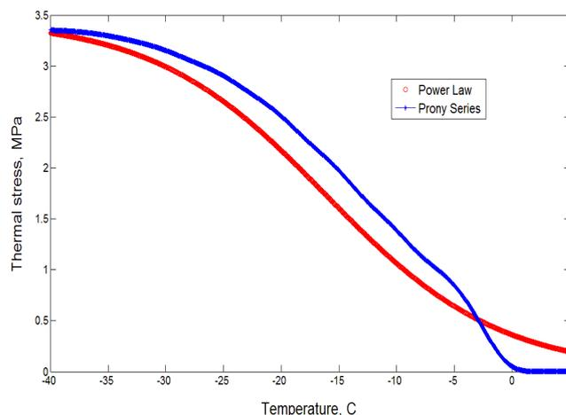
**Fig. 5.** Comparison of Thermal-induced Stresses between the Generalized Power Law and the Prony Series Functions.
