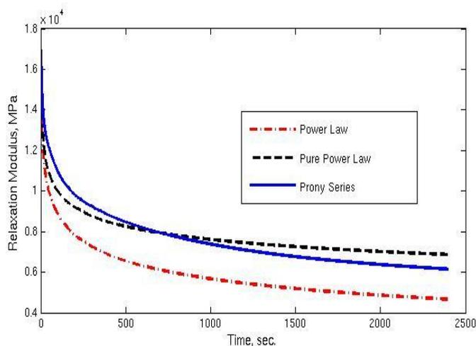
**Fig. 4.** Comparison of Relaxation Moduli between Three Representation Functions.
