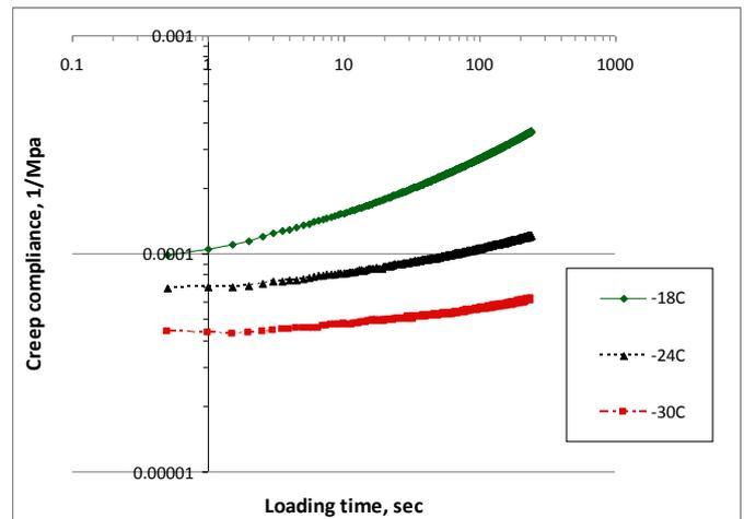
(a) Creep compliance curves at three temperatures
