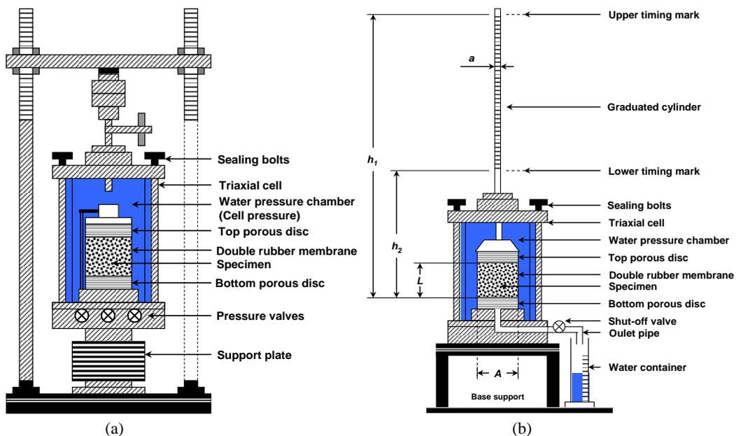
**Fig. 2.** Hydraulic Conductivity Tests: (a) Triaxial Cell for the Measure in Impervious Mixtures, and (b) Falling Head Test by Using Triaxial Cell and Graduated Cylinder for the Measure in Pervious Mixtures.
