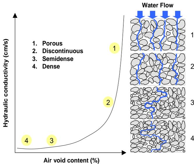
Fig. 4. Schematic Relationship between Hydraulic Conductivity and Air Void Content in Asphalt Mixtures with Different Pore Structure.
