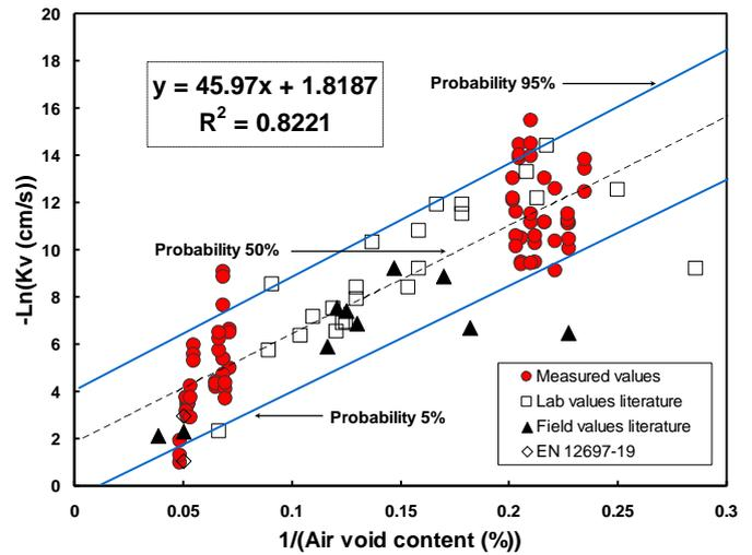
Fig. 6. Negative Logarithm of the Hydraulic Conductivity of Measured and Literature Values Versus Inverse of the Air Void Content.
