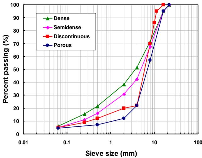
**Fig. 1.** Mixtures Graded Aggregates Distribution: Nominal Maximum Aggregate Size (NMAS) of 16 mm for Mixtures Type Dense, Semidense and Porous, and 11.2 mm for Discontinuous Mixture.
