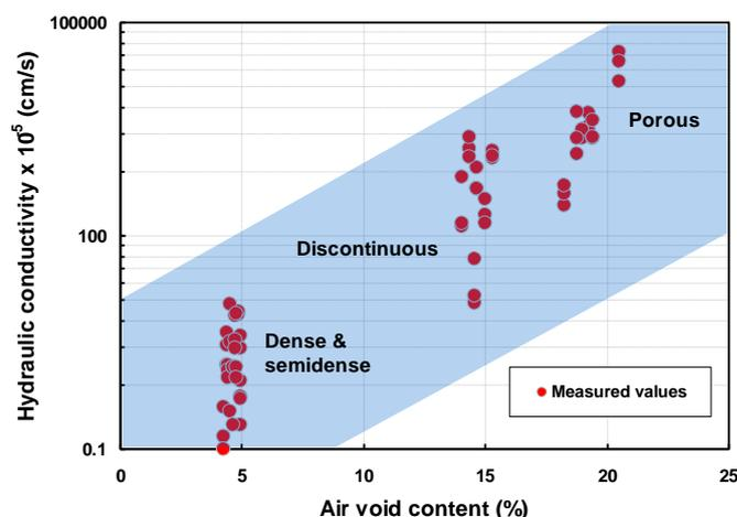
Fig. 3. Hydraulic Conductivity Versus Air Void Content of the Asphalt Mixtures Evaluated.
