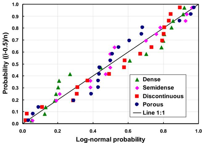
Fig. 5. Probability-probability Plot for the Hydraulic Conductivity Data of all Asphalt Mixtures Tested.
