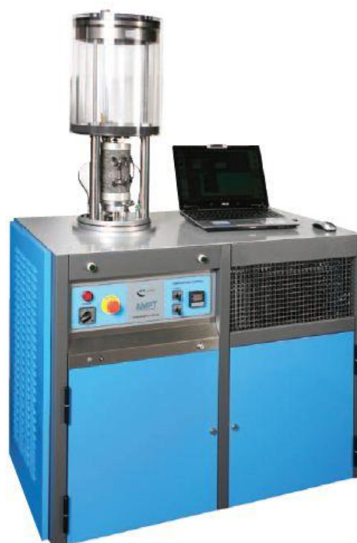
Fig. 1. Asphalt Mixture Performance Tester.
