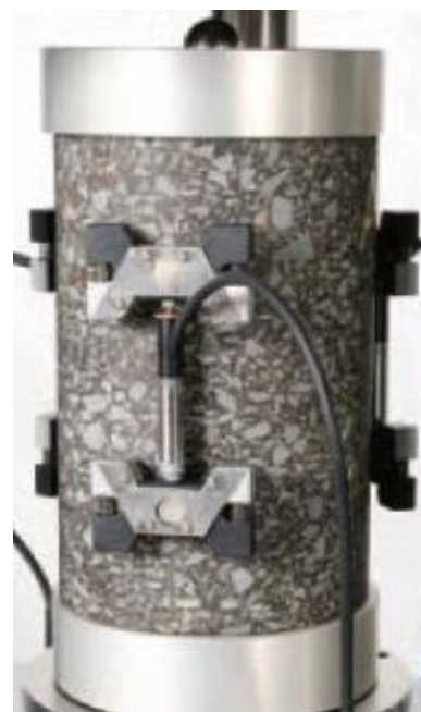
Fig. 2. HMA Specimen with LVDTs Attached for |E^*| Test with the AMPT.
